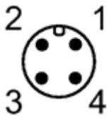
The flow monitor is equipped with a standard M12x1 connector with 4 pins.
