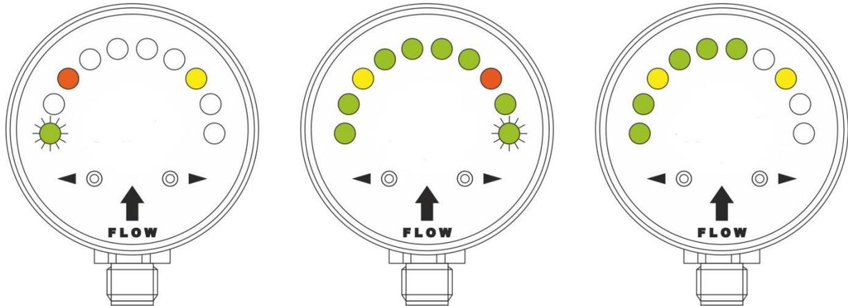
first LED flashing = the flow is below the monitor monitoring range
